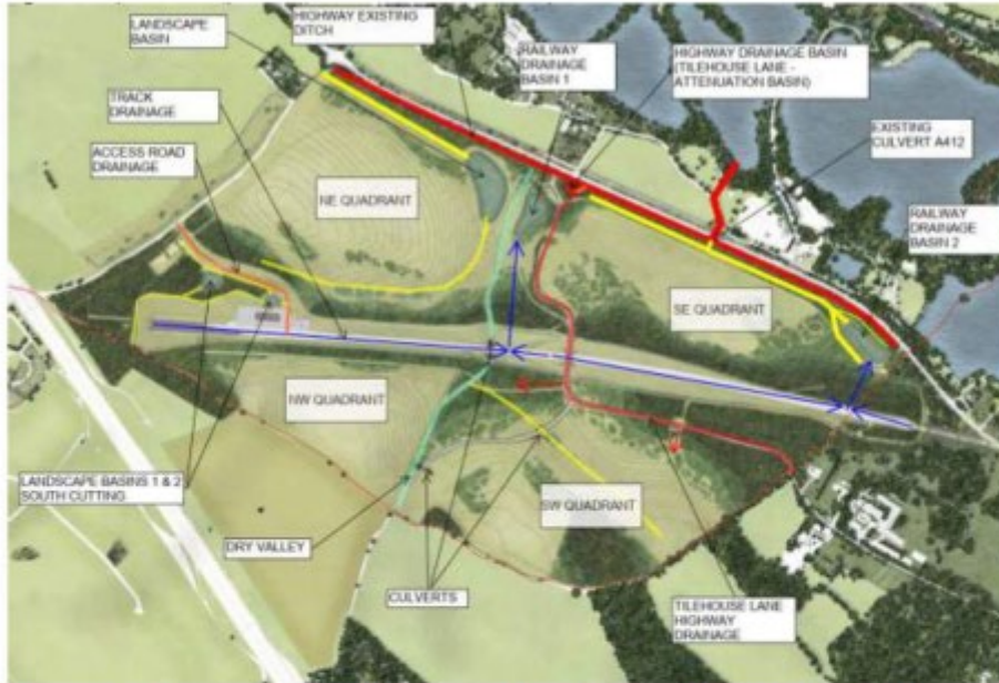
Figure 4: Drainage Strategy for Colne Valley Western Slopes. Written Statement. Application Ref: PL/21/0591
